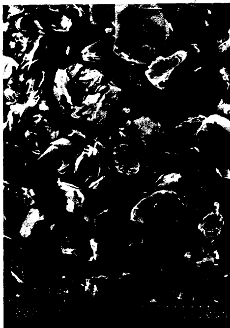
Fig. 7. Morphology of divided UF4 graphite observed by scanning electron microscopy.
