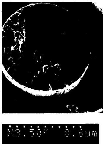
Fig. 5. Morphology of a graphitized P100 fibre observed by scanning electron microscopy.
